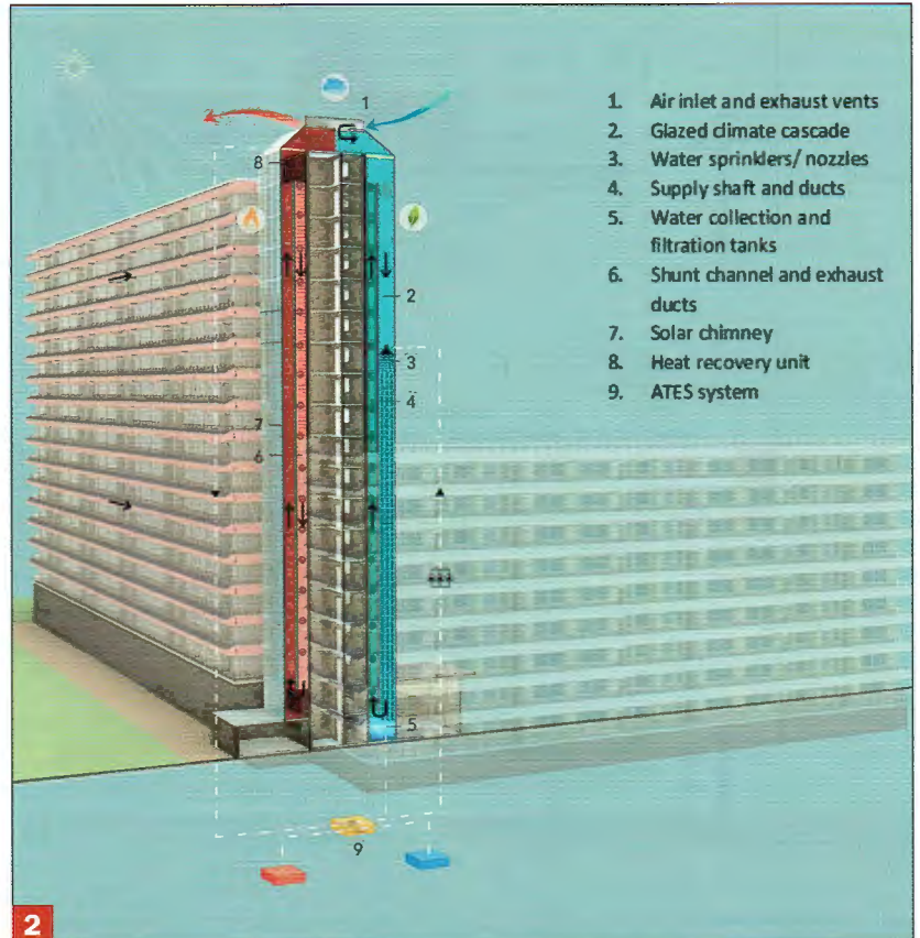
Vertical section through the building showing the integration of the EWF system
